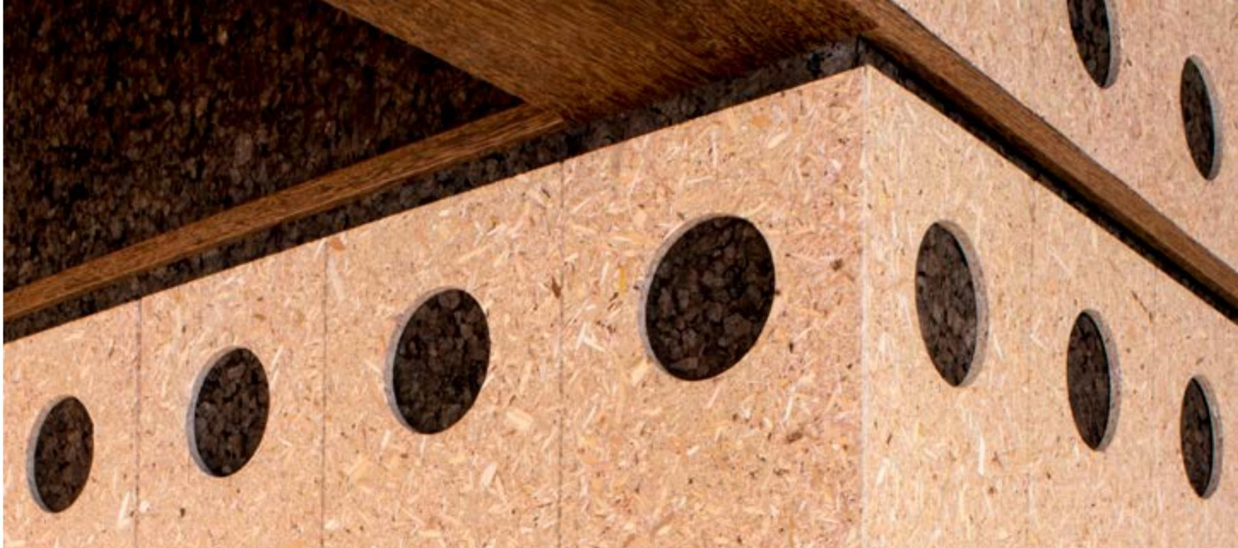
The board of wood particles is the pioneer of technical products derived from wood. Its incorporation into the market in the 40s of the last century made it possible to have panels in large size, with a flat and consistent surface, good mechanical resistance and dimensionally more stable than solid wood.
